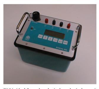
IRIS Instruments is pleased to introduce its new resistivity meter, SYSCAL Kid, a very compact unit specially designed for shallow electrical surveys. The SYSCAL Kid offers the well-known reliability and measurement accuracy of the entire SYSCAL range of resistivity meters.
