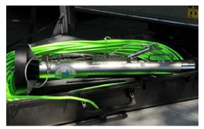
The sonar's role in this recovery highlights the benefits of its use: small size, usability, and effectiveness even in deep water. The equipment's powerful software, comparable to software found in more expensive systems, enables swift and accurate target identification through high resolution, real-time side-scan images.
